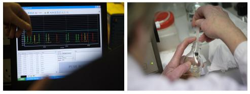
When creating whisky, it's crucial to quantify quality, consistency, and off-notes, faults or flaws. Technology such as Gas Chromatography Mass Spectrometry (GC-MS) can dissect a spirit into its many chemical parts. Yet despite such advances, nothing can analyse the quality of whisky quite like the human nose.
